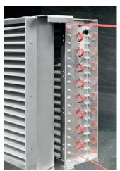
To separate droplets from the air H+R developed droplet separators made of PP, Aluminum or Stainless Steel. Our newest development is the electrical heated droplet separator with vanes made of aluminum elements and designed using CFD-analyseS.
